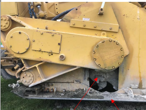
Void worker's foot and leg entered.
